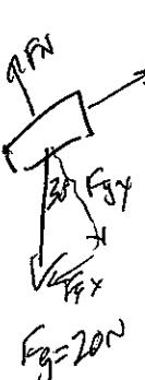
$$\begin{aligned} F_{gx} &= 20 \sin 30 = 10 \\ F_{gy} &= 20 \cos 30 = 17.3 \\ \text{since constant velocity, force cancel,} \\ \text{so } F_F &= F_{gx} \\ F_N &= F_{gy} \end{aligned}$$
