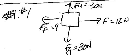
$$\begin{aligned} F_{\text{net}} &= ma \\ -(3)(9) &= 30a \\ a &= -3.06 \text{ m/s}^2 \end{aligned}$$
