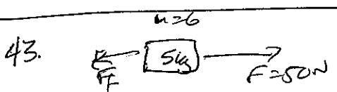
$$\begin{aligned} F_{\text{net}} &= ma \\ 50 - F_f &= 5(6) \\ F_f &= 20 \text{ N} \end{aligned}$$
